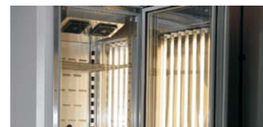
FIT DS - light tubes installed in door and side walls
