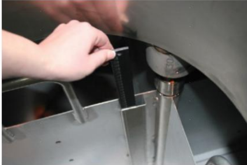
Level dip stick inserted to measure the physical liquid nitrogen level
