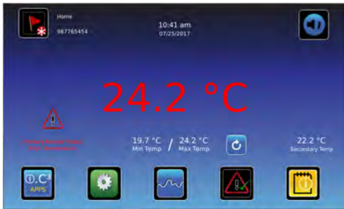
Home screen with active alarm
