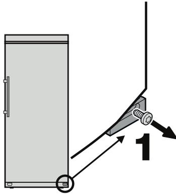
5. Turn lower hinge pin through 180° and remove.
