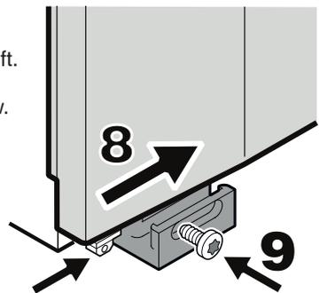
4. Transfer lower hinge bracket and cover plate to the opposite side.
