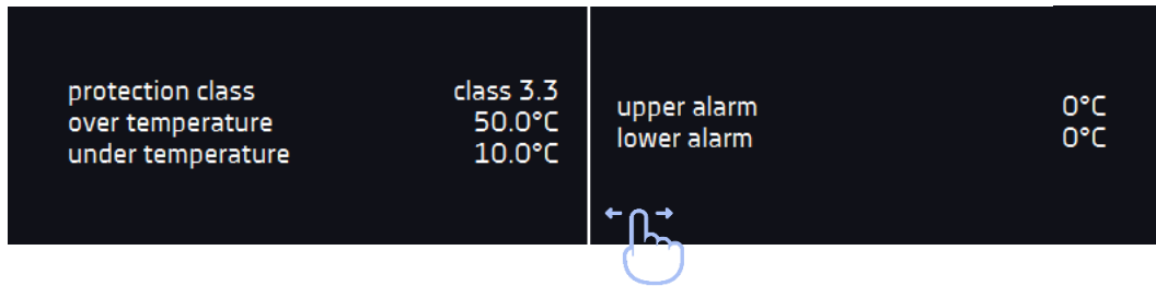
Figure 11 Status – protection and alarms
