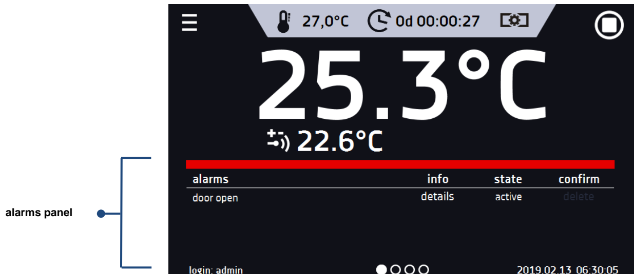
Figure 9 Icon: Alarms panel
