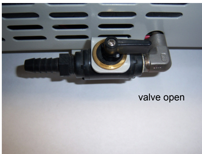
Figure 6. Drain valve open
