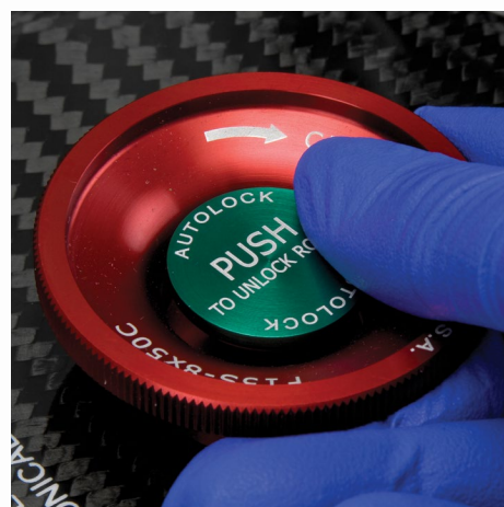
Figure 13. Easy and secure push-button Auto-Lock rotor exchange in as little as 3 seconds for application versatility and cleaning convenience.
