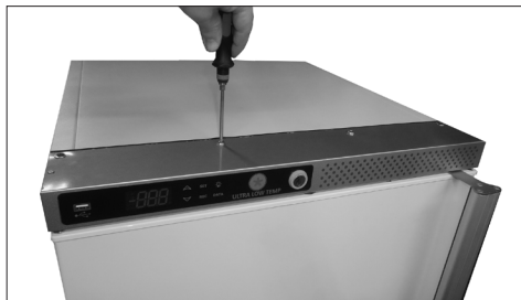
44. Remount the four topscrews
