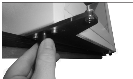
30. Remount and tighten the two front feet
