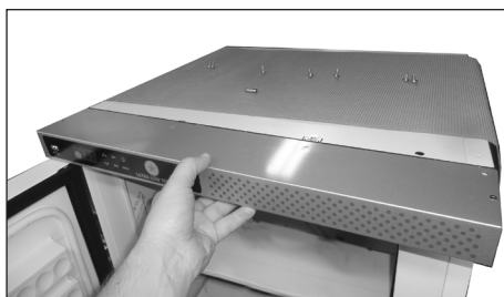
40. Carefully push the toppanel back into position
