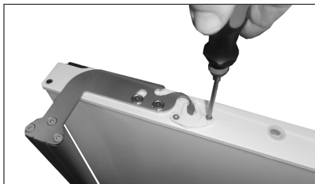
37. Remount the two screws and the door-closer is fixed
