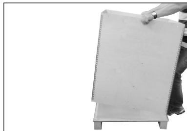
5. Remove box and lift down the appliance
