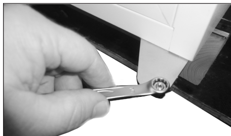
24. Remount and tighten pivot nut
