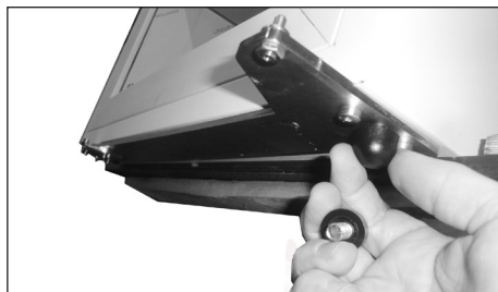
18. Remove the two front feet
