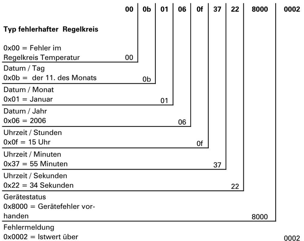
**Figure 12-46.** Error memory data set structure
