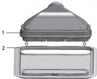
**Figure 4-6.** Mounting the airbox on the water reservoir cover
