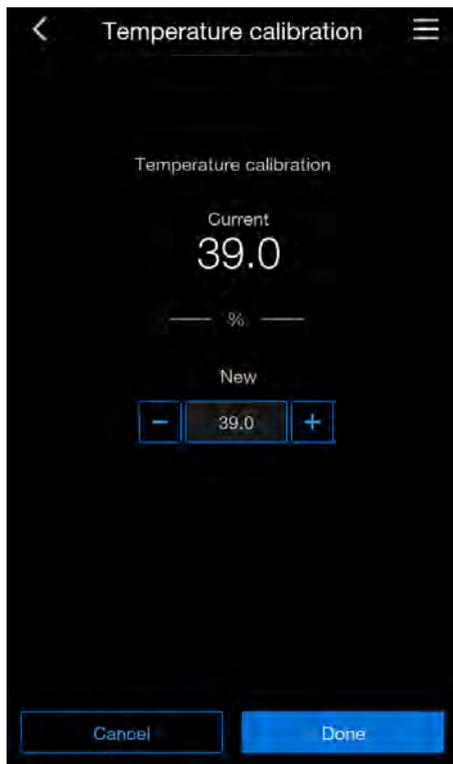
**Figure 9-3.** Performing the temperature calibration
