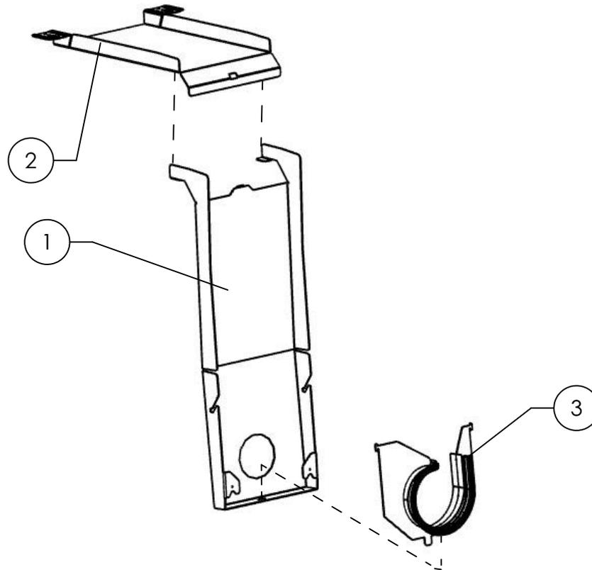
Figure 4-3. Air duct parts Vios iDx 165/255
