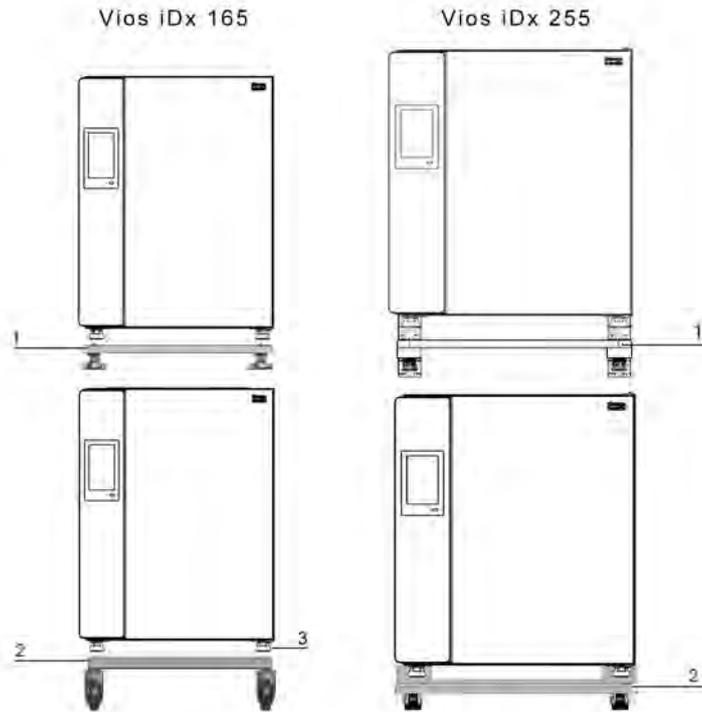
**Figure 2-3.** Stacking devices
