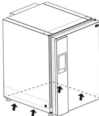
Figure 2-2. Lifting points
