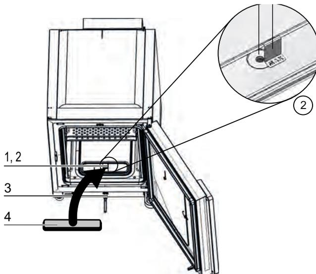
Figure 4-2. “MAX” Fill Level Indicator and pre-filter
