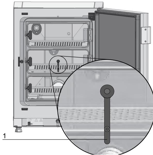
**Figure 9-4.** Measurement opening in a segmented inner door
