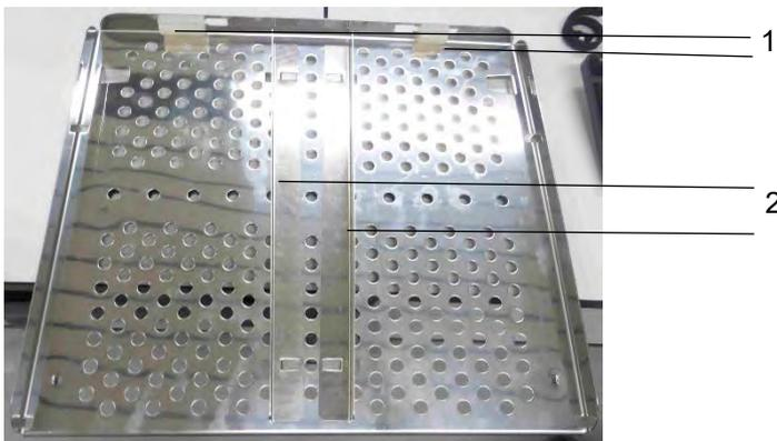
**Figure 14-3.** Perforated shelf with continuous guide rails
