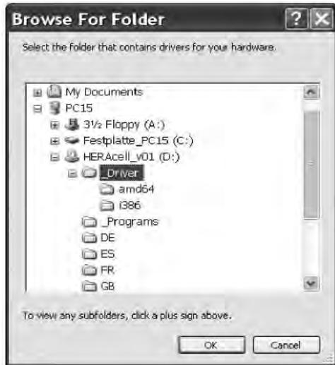
**Figure 12-45.** Installing the USB interface driver - 4
