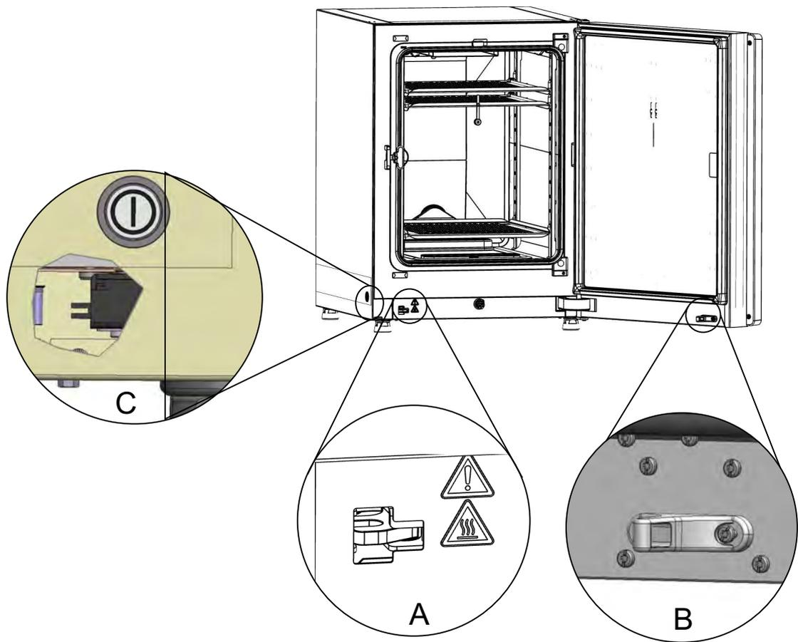
**Figure 3-16.** Door lock lever and emergency release
