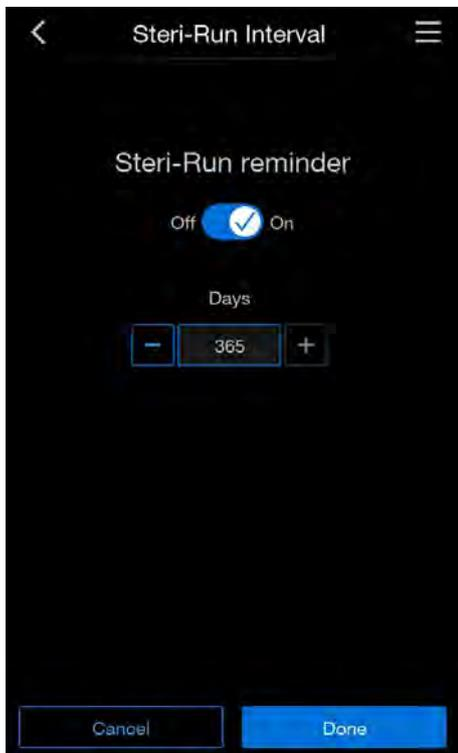
**Figure 6-33.** Setting the reminder interval for Steri-Run
