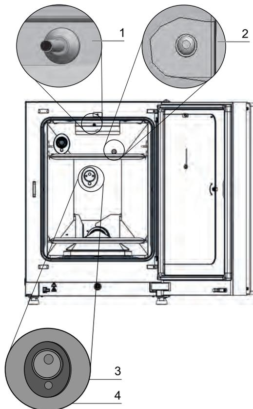
**Figure 3-6.** Temperature, O<sub>2</sub>, CO<sub>2</sub>, and humidity sensors
