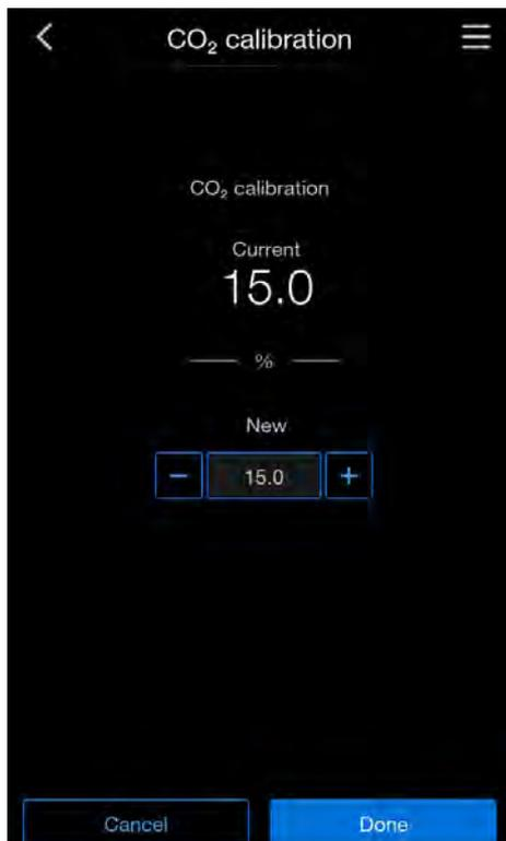
**Figure 9-6.** Performing CO<sub>2</sub> calibration
