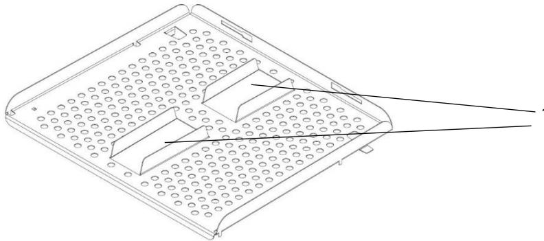
**Figure 14-4.** Perforated shelf with divided guide rails (below)
