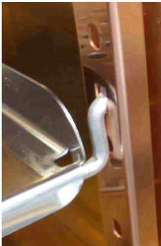
**Figure 14-5.** Installing the perforated metal shelf
