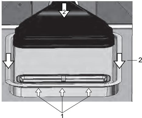
**Figure 9-7.** Removing the airbox
