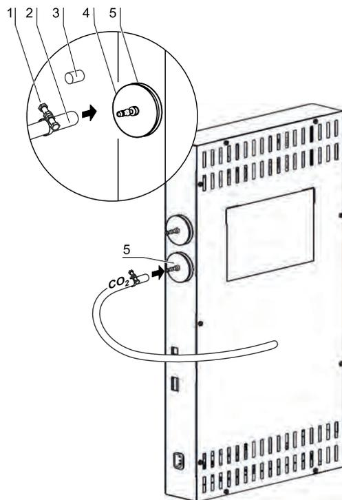
**Figure 4-11.** Installing gas pressure hoses
