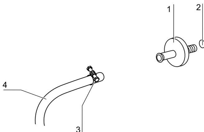
**Figure 9-9.** Gas intake filter installation
