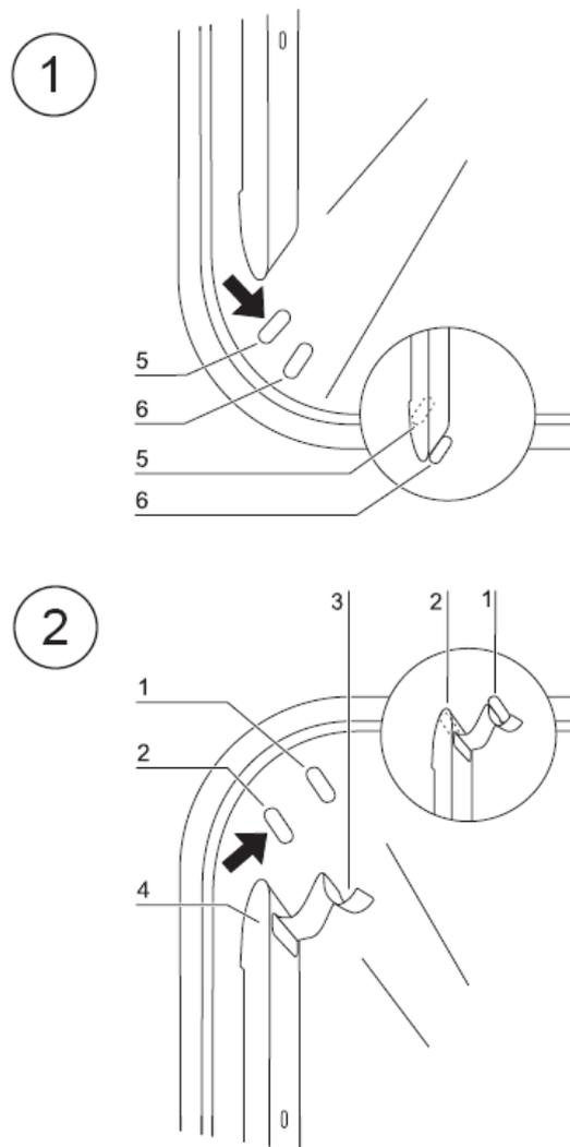
**Figure 4-8.** Shelf system installation/removal
