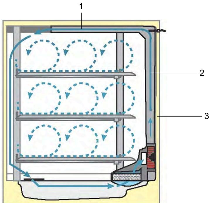
**Figure 3-4.** Air duct
