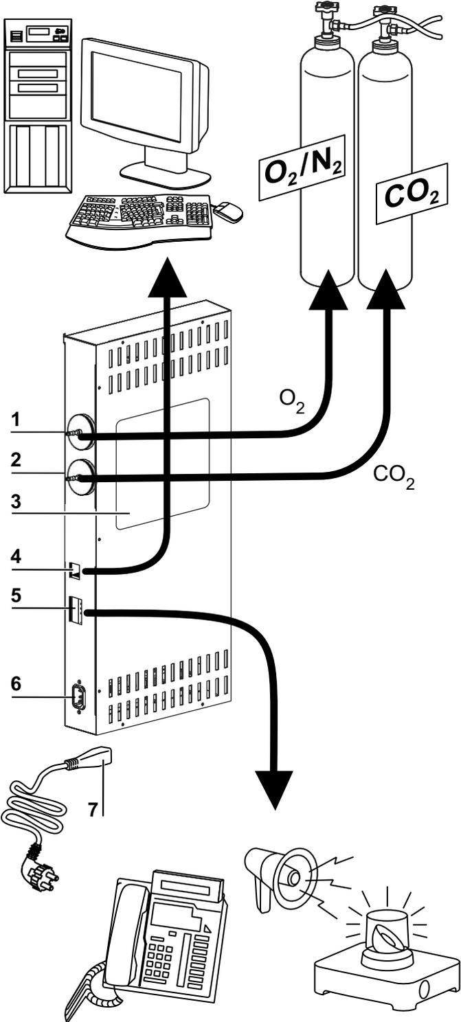
Figure 3-8. Device interfaces (right side of control box)
