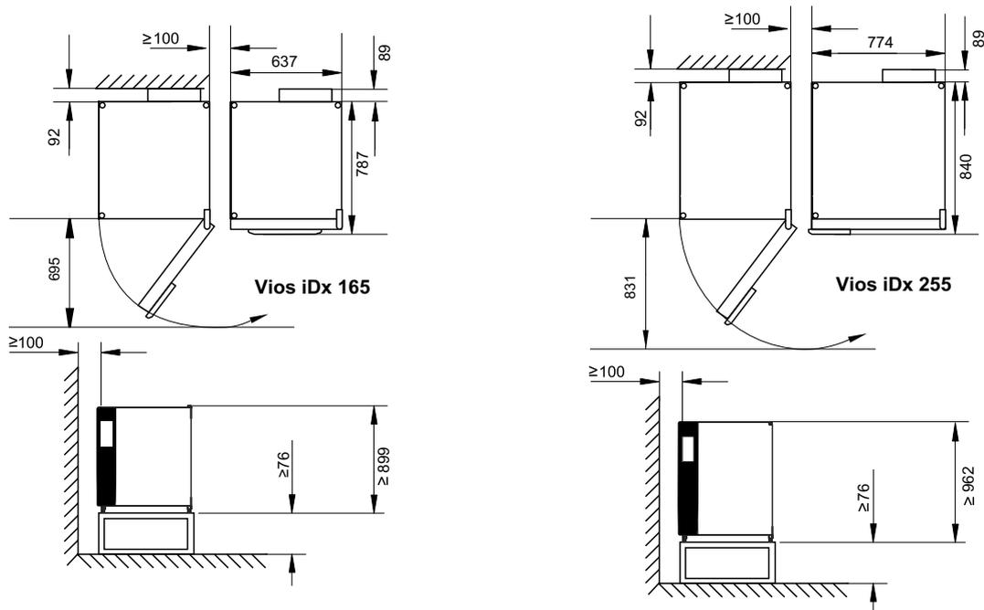
**Figure 2-1.** Device measurements (All dimensions in mm)
