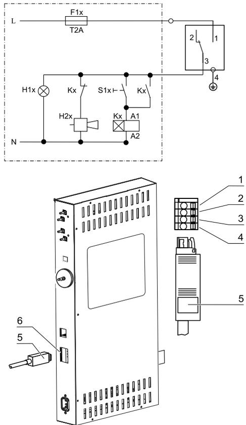
**Figure 4-14.** Example of alarm contact connection
