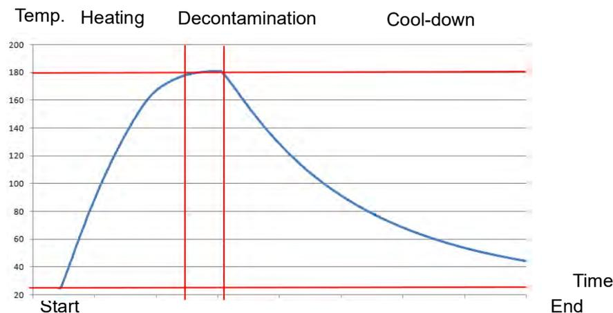
Figure 8-4. Phases of the Steri-Run sterilization cycle
